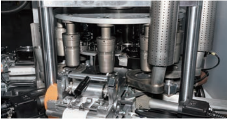
杯底三道热风 TRIPLE HOT AIR
