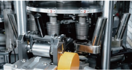
杯底三道热风 TRIPLE HOT AIR
