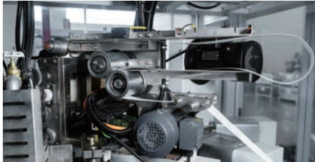
一体式冲底成型机构 INTEGRATED BOTTOM PUNCHING MECHANISM
