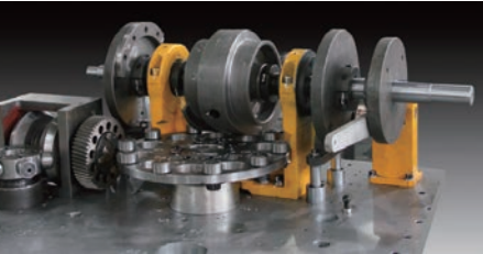
双分度凸轮 DOUBLE INDEXING CAM ASSEMBLY
