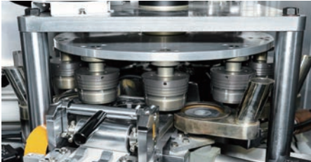
杯底三道热风 TRIPLE HOT AIR
