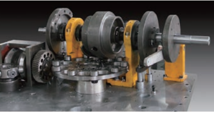
双分度凸轮 TWO INDEXING CAMS ASSEMBLY
